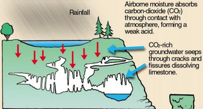
Airborne moisture absorbs carbon-dioxide (CO<sub>2</sub>) through contact with atmosphere, forming a weak acid.
